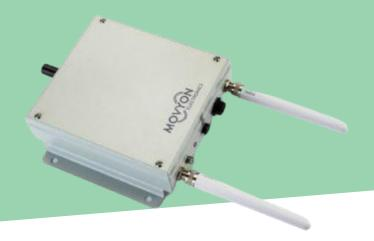
The Road Side Unit C-ITS enables two-way wireless communication between the roadside infrastructure and the On Board Unit (OBU) in the vehicle, ensuring high levels of safety and reliability in data exchange. IT enables advanced monitoring of roadside events and efficient traffic management. The solution, fully developed and manufactured by Movyon Electronics, can be customized according to customer needs.
