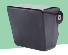
Movyon Electronics 24.0 GHz FMCW (Frequency Modulated Continuous Wave) radar, exploiting the Doppler effect and continuous frequency modulation, allows to reliably detect the instantaneous speed and distance to the antenna of moving vehicles. Resistant to even the most extreme weather conditions, this radar can identify the transit, direction and class of vehicles moving between 30 and 300 km/h, with an accuracy of over 97%.
