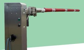
A patented quick-acting barrier with the ability to automatically reposition the rod in the event it is hit by a passing vehicle, either in the direction of normal travel or in the opposite direction. Particularly suitable for use in applications such as motorway toll booths and parking lots, it is designed with sturdy and impact-resistant satinized stainless-steel cabinet. The barrier meets special requirements such as a high number of cycles and a high speed of maneuvering.
